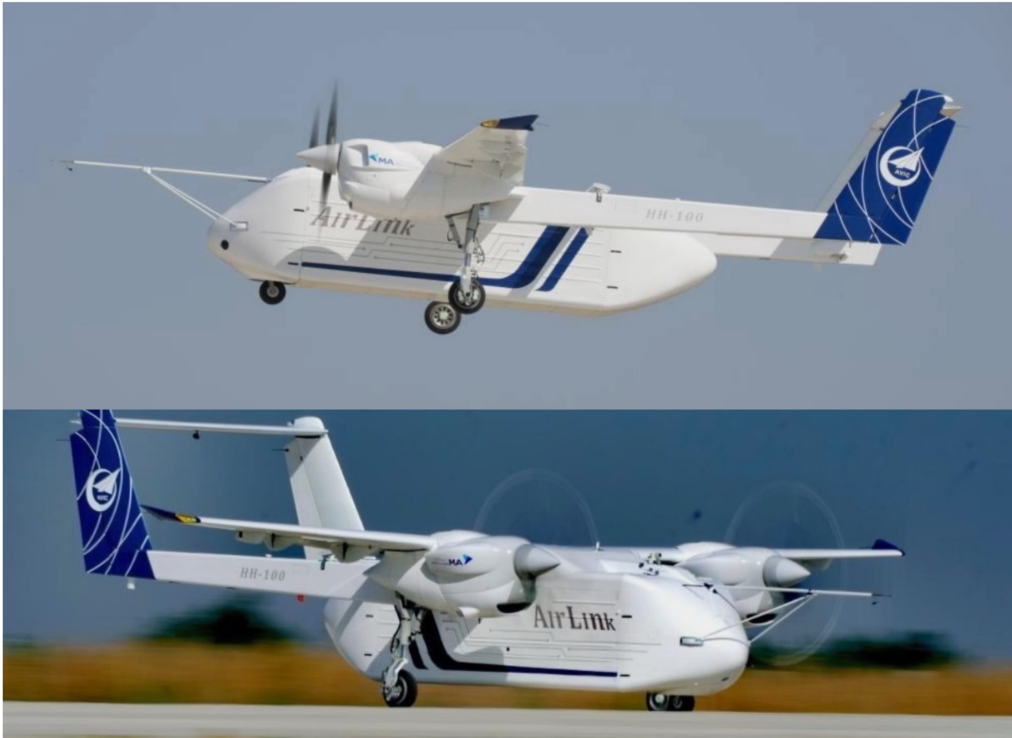
Un-manned transport airplane HH-100 of Aviation Industry Corporation (AVIC) on its first flight at the airport of Xi'an.
